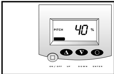
**IMPORTANT: Changes to the power level settings can only occur when the compressor is not running. Pressing any button when the compressor is running, activates an emergency shut down.**
