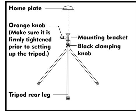
5. Set the tripod upright. If the legs wobble, loosen the black knob and reset the legs. Firmly tighten the black knob until the legs are secured.
