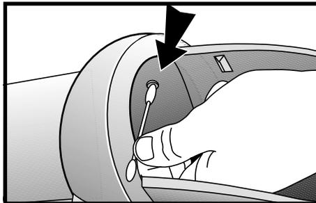
The optical sensors that detect the ball and measure its speed are located in the orange plastic recesses on opposite sides of the barrel just inside the ball scoop. Clean the sensors with a moist cotton swab.
