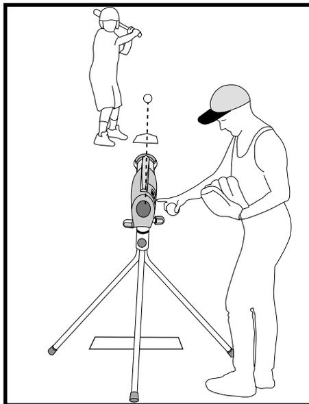
To adjust the pitch height in the strike zone, slightly increase or decrease the power level. If the power level is changed significantly, you will need to adjust the pitch angle (elevation). Refer to “Determining the Pitch Angle” on page 9.
