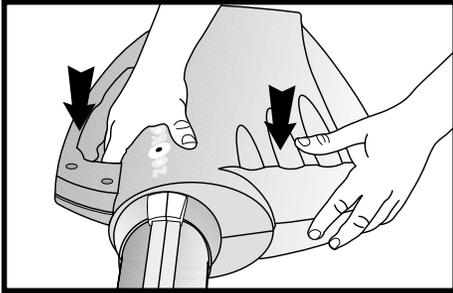
12. Replace the top of the case and align the mounting holes. If it is properly aligned, you will hear a click as you apply gentle pressure to the top of the case.
