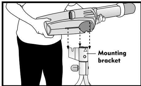
Take the following steps to assemble the machine onto the tripod:
