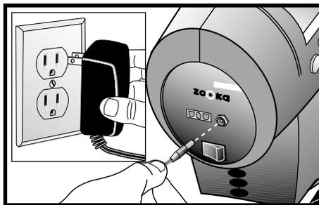
During long-term storage, the battery should remain permanently connected to the charger and the charger plugged into a power source. A microprocessor, inside the machine, monitors the battery and maintains a full charge.
