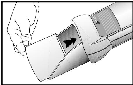
5. Wipe off the cup and remove any embedded grit or gummy buildup. If necessary, scrape carefully with a putty knife or other dull blade. Wash the cup in a mild solution of dishwashing liquid and water.
