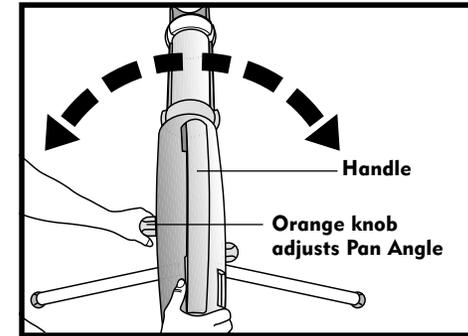
1. Hold the machine's handle while loosening the orange knob on the tripod's mounting bracket one full turn. See Diagram 12.
