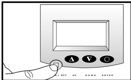
**NOTE:** To turn the machine OFF, press the ON/OFF button. The machine beeps twice and turns OFF.
