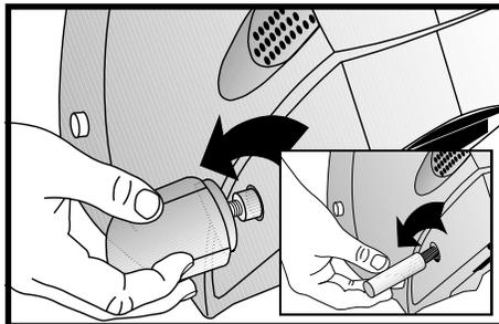
4. Hold the machine by its handle and remove the orange knob by rotating it counterclockwise. Set the knob aside. See Diagram 28.
