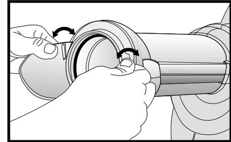
3. When the cup reaches the ball scoop, you will need to pull the rubber away from the sides of the cup to facilitate removal.
