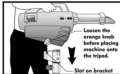
2. Loosen the orange knob on the machine so that it is easy to mount the machine onto the bracket.
