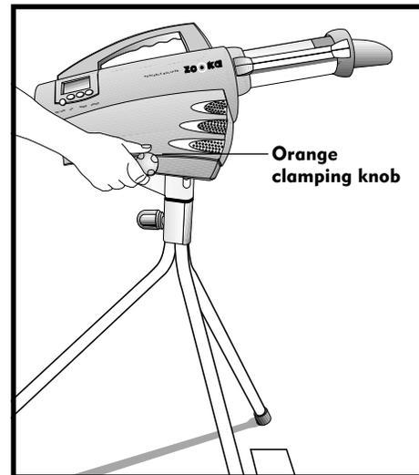
**NOTE:** It may help to wiggle the machine slightly to seat the clamping bolt in the slot on the tripod's mounting bracket.
