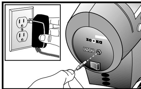
3. Plug the end of the charger cable into the rear panel. See Diagram 5.
