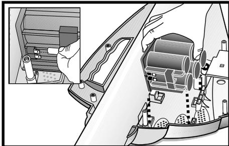
9. Remove the battery connectors. Gently, slide both wire connectors off of the old battery. Pull on the connectors, not on the wires.
