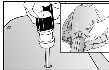
7. Remove the 10 screws with a Phillips head screwdriver. Set the screws aside.
