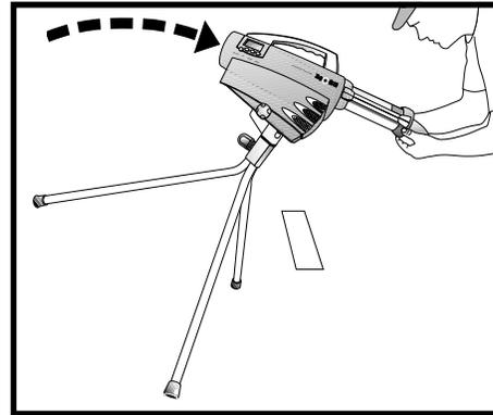
**NOTE:** If the cup is out of reach, position the machine so that the barrel faces down. Gravity helps the cup settle forward.
