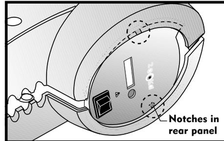
**IMPORTANT:** Check that the rear panel is properly positioned prior to replacing the case. Do not tighten the screws until the rear plate is secure. The two notches in the rear panel align it properly. See Diagram 32.
