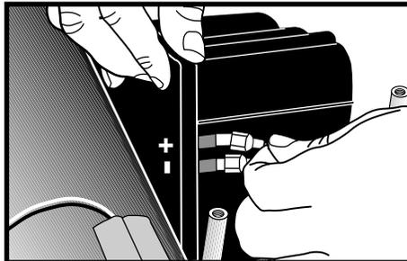
11. Replace the wire connectors. Connect the red wire to the + terminal. Connect the black wire to the - terminal.
